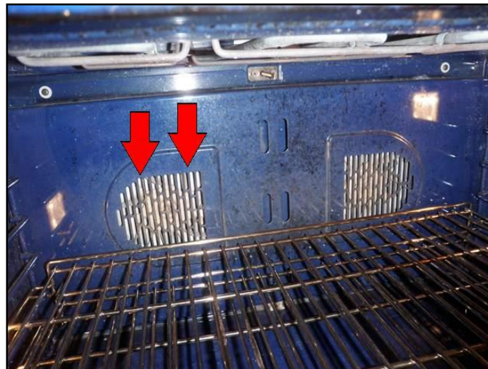
Noisy fan- blade hits housing
