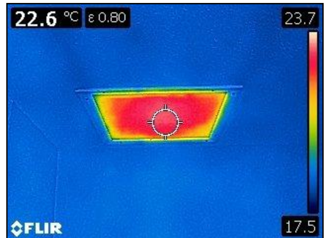
35. Not insulated and not weatherstripped
