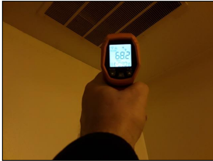
Heater return temp 68 deg
