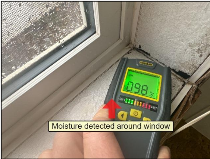
65. Moisture detected around window
