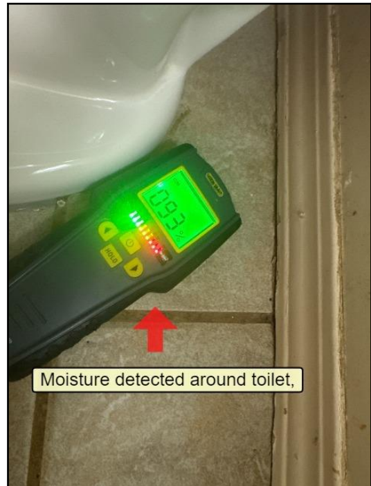
58. Moisture detected around toilet,
