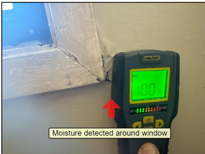
63. Moisture detected around window
