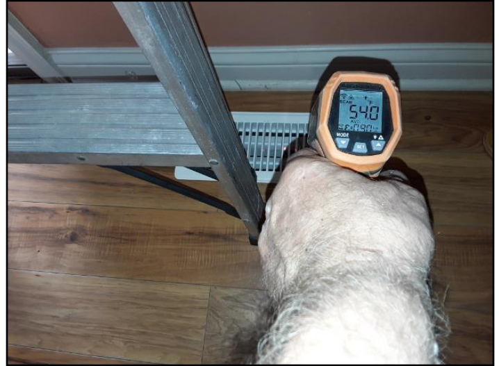
32. Cooling supply temp 54 deg
