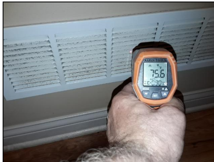
33. Cooling return temp 76 deg
