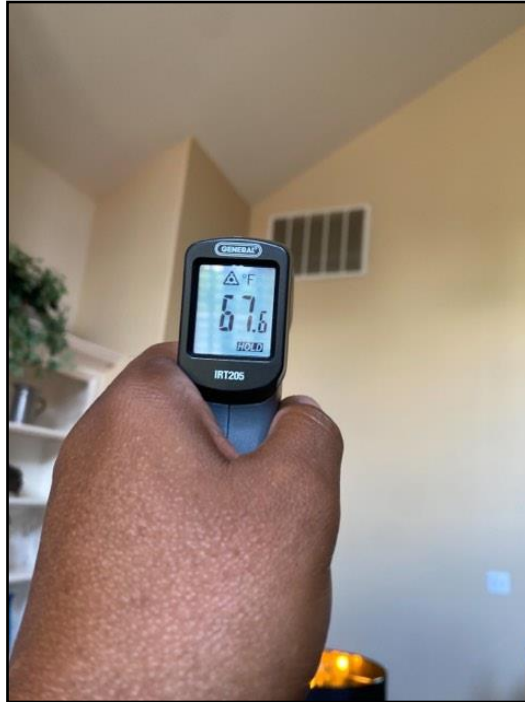
51. Temperature split across cooling coil less...
