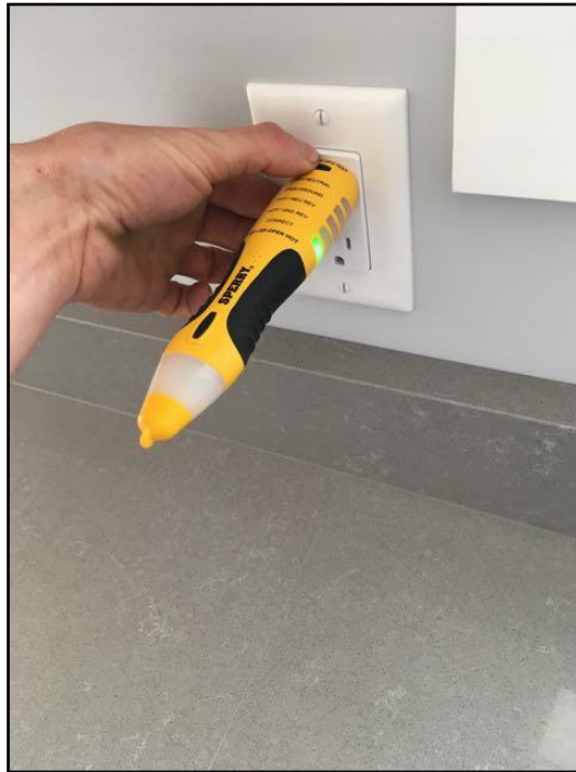
No GFCI/GFI (Ground Fault Circuit...
