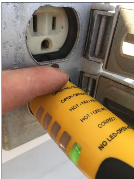
No GFCI/GFI (Ground Fault Circuit...
